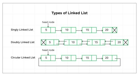
When a node contains a pointer storing the address of the next node, the list is called a **singly linked list**. When a node contains two pointers storing the address of the previous node and the next node respectively, the list is called a **doubly linked list**. When the list is found to be circular, the list is called a **circular linked list**.
